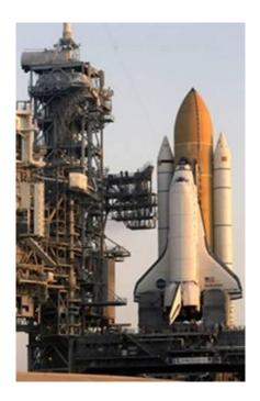
The engineers who designed the SRBs would have preferred to make them a bit larger, but the SRBs had to be shipped by train from the factory to the launch site. The railroad line from the factory happens to run through a tunnel in the mountains, and the SRBs had to fit through that tunnel. The tunnel is slightly wider than the railroad track, and the railroad track, as you now know, is about as wide as two horses' behinds.
