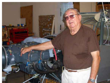
John is plugging away on his Super Cruiser, he is working on the engine baffling right now.
